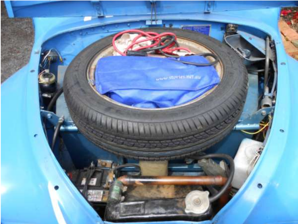
More fiddling to fit things in but note neat fit of Mini radiator (& compliance plate at rear)
