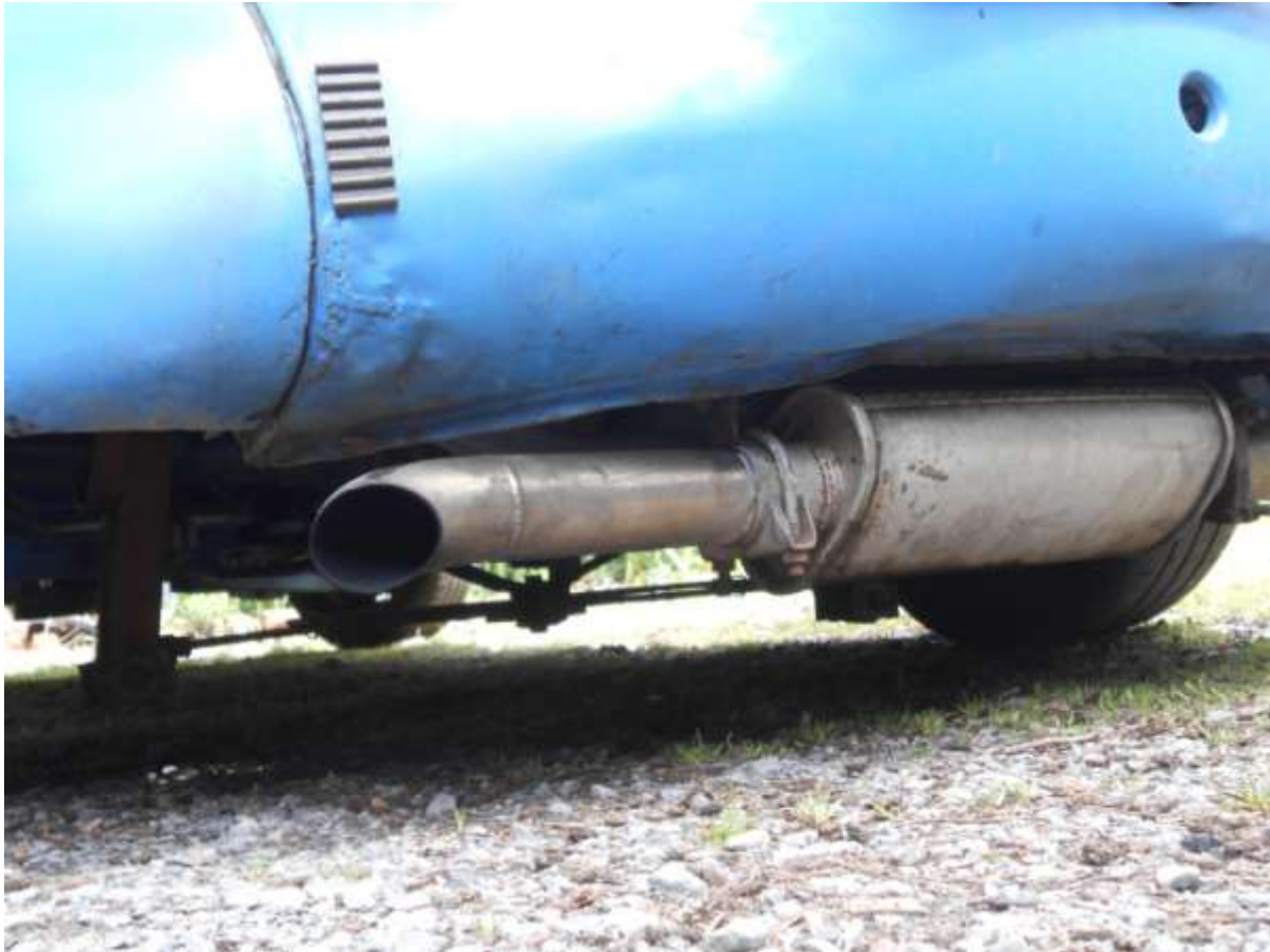
Camber compensator & a too-low "muffler"
